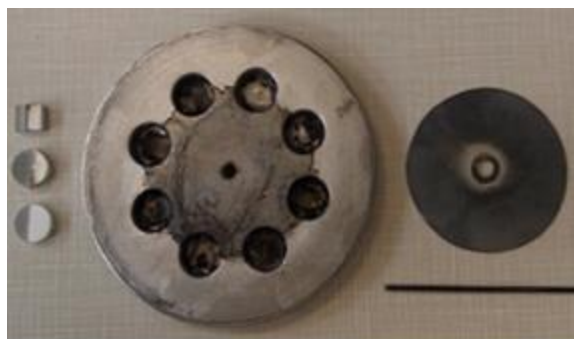
Figure 2.1 The magnetron sputtering target. The sputter material is replaced with the sample holder (left) with a shadow shield that covers half the exposed sample face (right).
