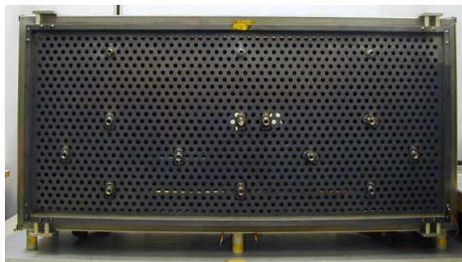
Figure 3-8: Photograph of the MCDC ion collection grid showing the button probe locations.
