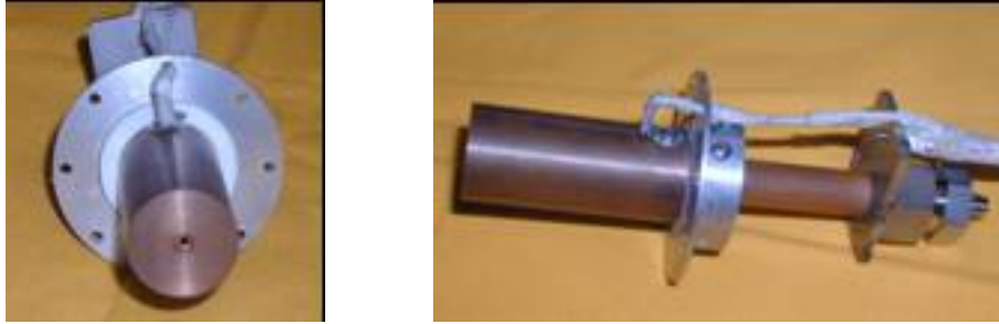
Figure 3-3: Photographs of the dormant cathode units (DCUs).
