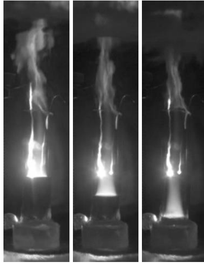
Fig. 6. High-speed images of nitromethane decomposition
