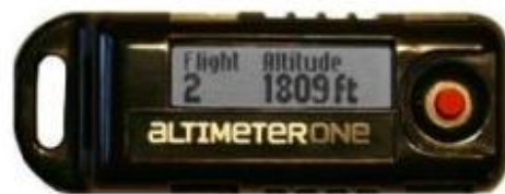
Figure 5: Jolly Logic AltimeterOne
