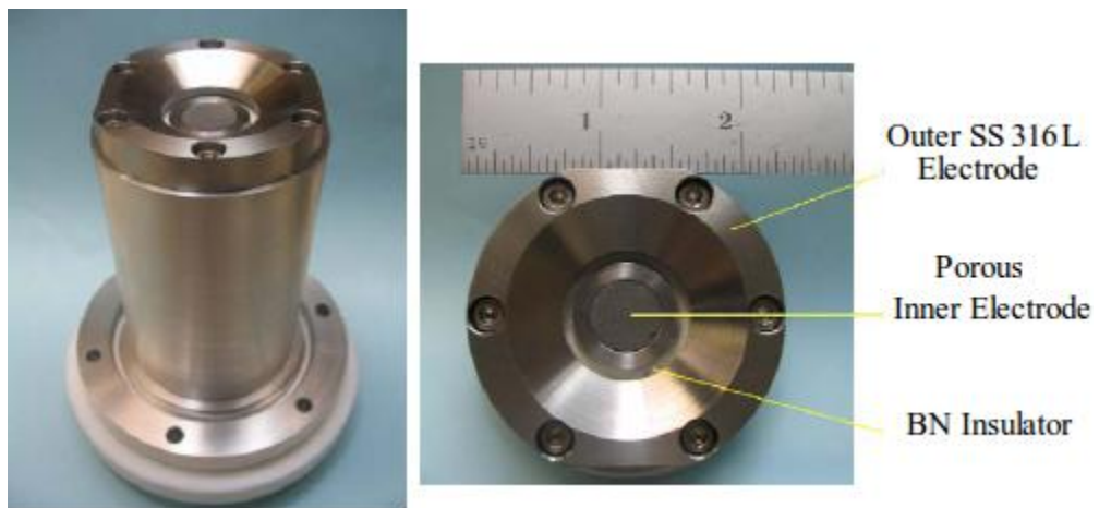
Figure 3.9: Photograph of coaxial gallium injector with a porous tungsten center electrode.
