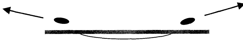
Figure 1.8 Sketch of macroparticle flight from a cathode spot
