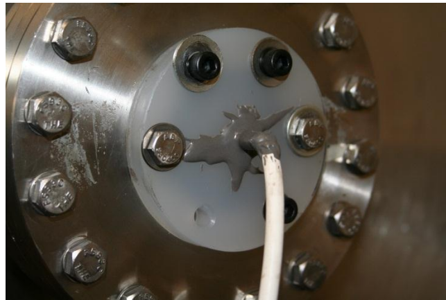
Figure B.1: The custom made high voltage pass-through used for high altitude testing.
