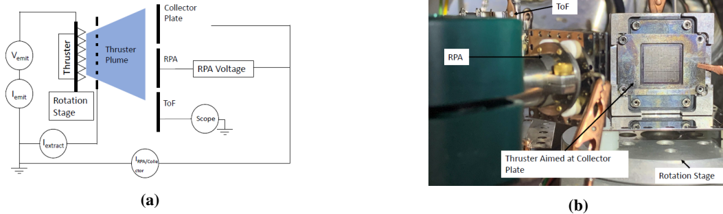
Fig. 4 Image of (a) the experimental set up diagram (b) the thruster mounted to the rotation stage inside of the vacuum chamber.
