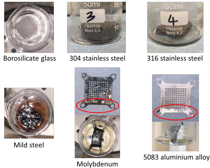
Fig. 3 Materials after two months of compatibility test with FAM-110A ionic liquid.
