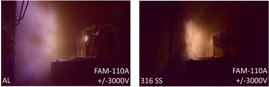
(a) Aluminum plate using FAM-110A, with the thruster pitch angle of -45 degrees. (b) Porous 316 stainless steel plate using FAM-110A, with the thruster pitch angle of 0 degrees.
