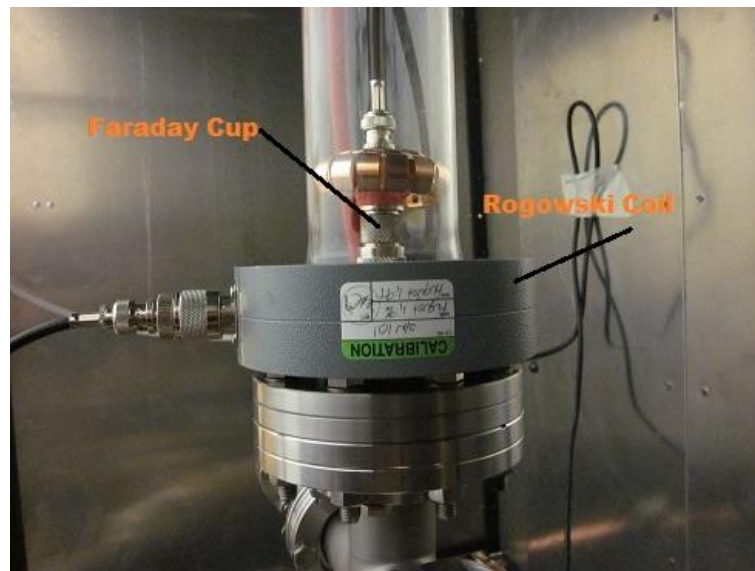
Figure 2.15. Faraday cup and Rogowski coil for electron beam detection
