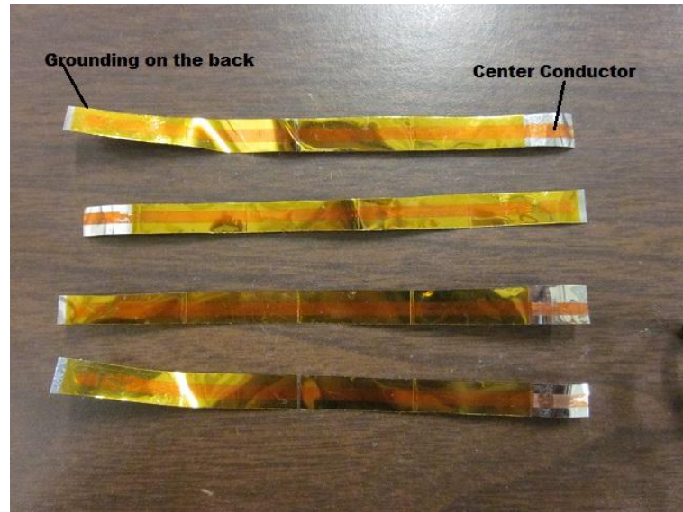
(a) Capacitive probes constructed on flexible PCB film
