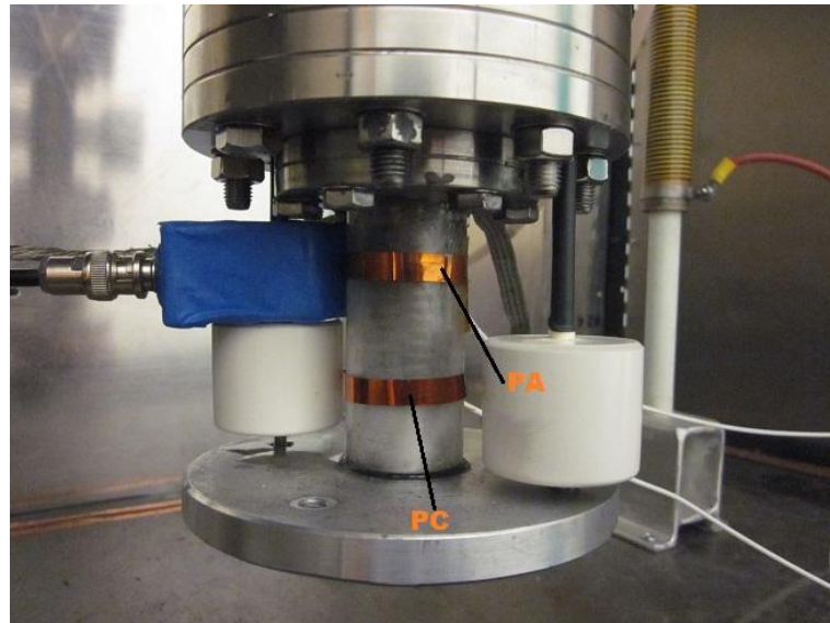
(b) Pseudospark chamber with two capacitive probes
