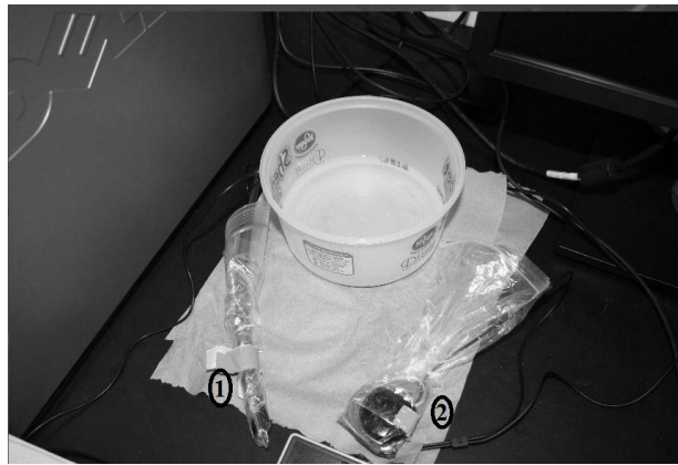
Figure 2.2. Headphone(1) and microphone(2) with waterproof 'enclosures'
