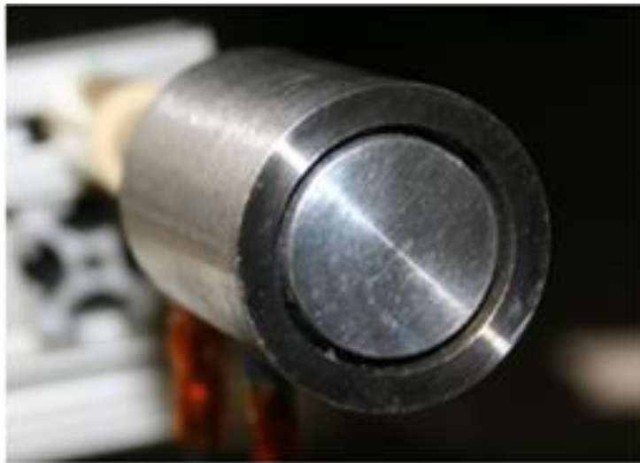
Figure 2.1. The APLab's NFP mounted in the vacuum facility [27].
