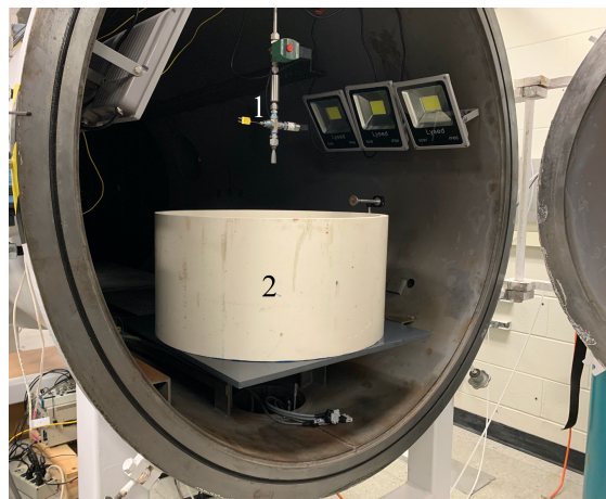
Fig. 4 Details of the PSI facility showing the cold gas thruster (1) and granular media bed (2).
