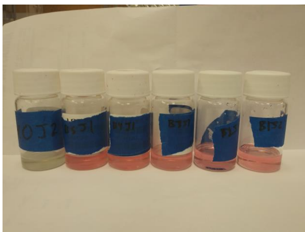
Figure 16. Photograph of 90% wt. HAN + water samples no additive, 0.05%, 0.1%, 0.5%, 1%, and 5% Bipy respectively, from left to right.
