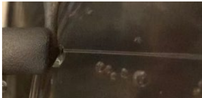
Figure 3. Water jet from the nozzle of thruster B2.
