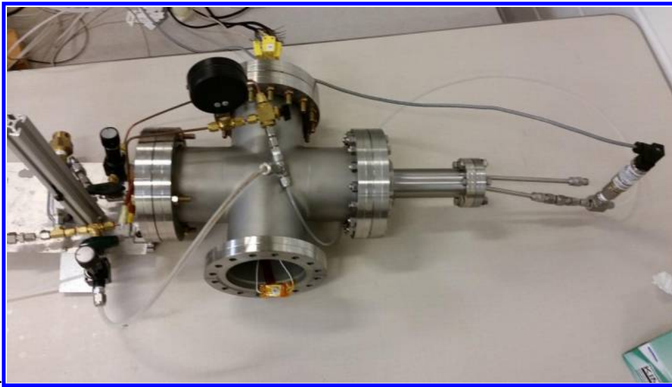
Figure 1. Photograph of the Batch Reactor Experiment in the Lab Showing Atmosphere Control Panel (left), Sample Holder (bottom), Pressure Measurement (right), and Temperature Measurement (top).
