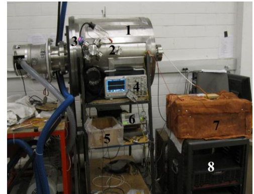
Figure 8. 1. Vacuum Chamber; 2. BNC-BNC Passthrough; 3. Lesker Pressure Gauge; 4. Tektronix DPO 2024 Oscilloscope; 5. Op-Amp Integrator Circuit; 6. Rigol Function Generator; 7. Faraday Cage; 8 High Voltage Probe
