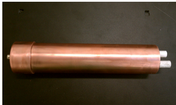
Figure 6: Finished voltage divider for high voltage output from flux loops
